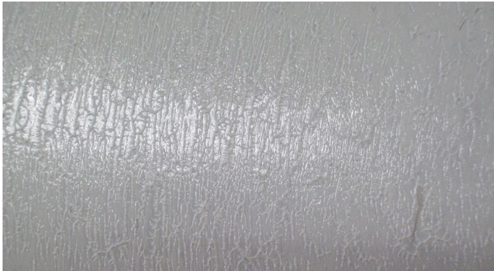
Figure 9 – Example of thermal paste residue on mounting plate
