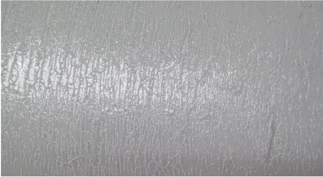
Figure 11 – Thermal Compound after removing controller
