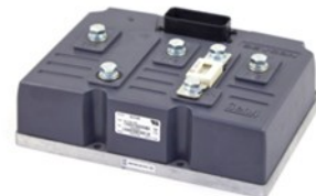
Sevcon Motor Controller
